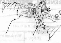
Fig. RA-28 Tightening Side Yoke Fitting Bolt
