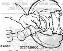
Fig. RA-16 Removing Grease Seal and Inner Bearing
