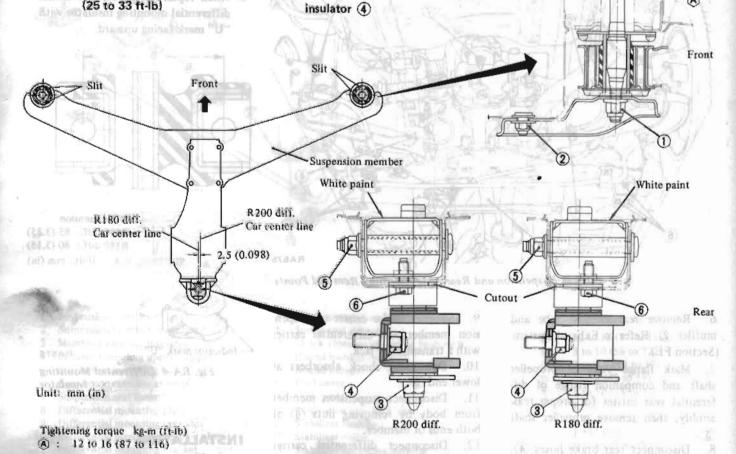
Note: Differential mounting bracket and adapter plate of R200 differential carrier are installed opposite to those of R180 differential carrier. Install them according to identification marks shown in table below.
