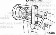
Fig. RA-7 Removing Insulator from Suspension Member
