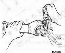
Fig. RA-22 Removing Yoke Flange
