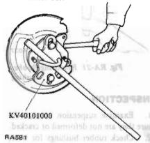
Fig. RA-14 Removing Wheel Bearing Lock Nut
