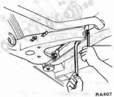
Fig. RA-20 Removing Suspension Alfandw Inori Xion Arm
