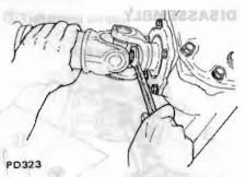
Fig. RA-23 Removing Side Yoke Fitting Bolt
