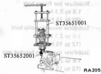
Fig. RA-10 Compressing Spring
