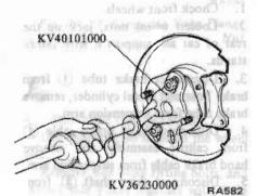
Fig. RA-15 Removing Rear Axle Shaft
