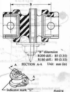
Fig. RA-4 Differential Mounting Insulator
