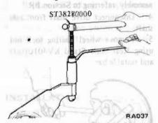
Fig. RA-21 Removing Rubber Bushing
