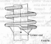
Fig. RA-12 Installing Coil Spring
